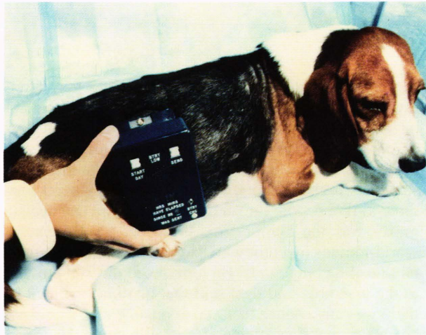
Figure 18. A patient programming unit being used to adjust insulin delivery in a diabetic test animal.
