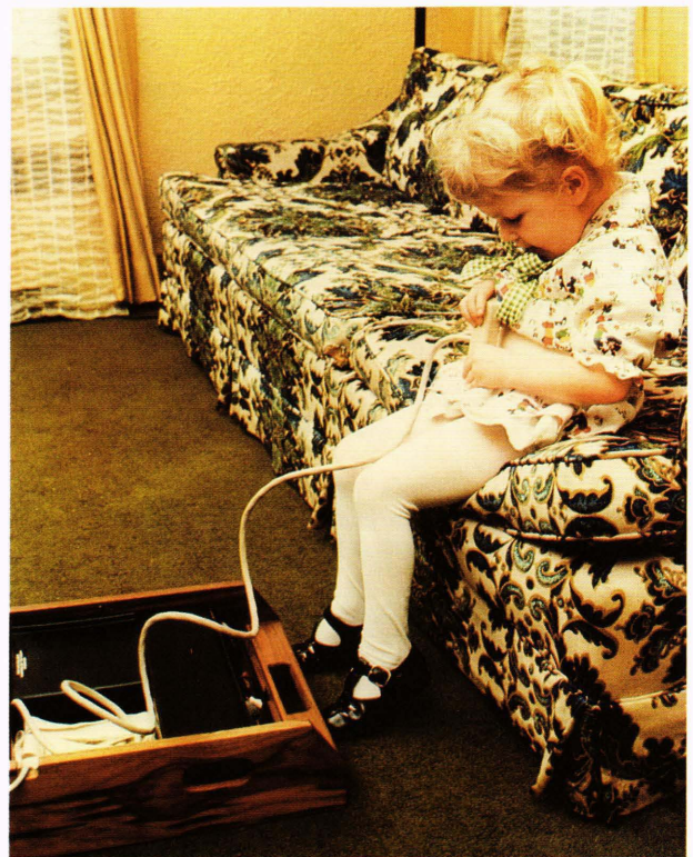
Figure 8. A three-year-old with a pacemaker implanted in the abdomen doing her own recharging.
