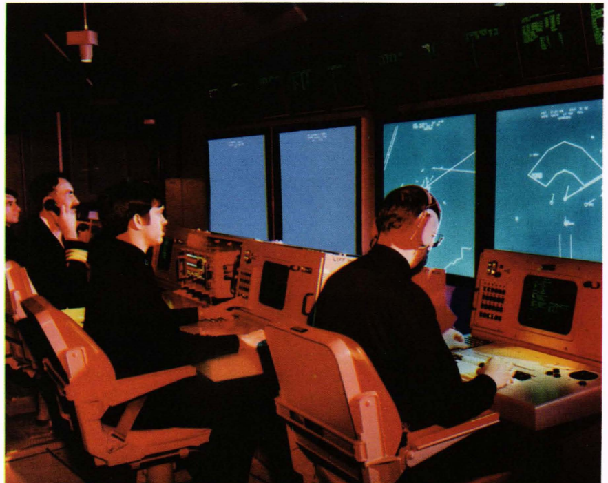
Figure 18. The Aegis display system. The complex system includes computer-driven large-screen displays, automated status boards, communication facilities, computer-control consoles, and a computer that is linked with shipboard weapons and sensors.
