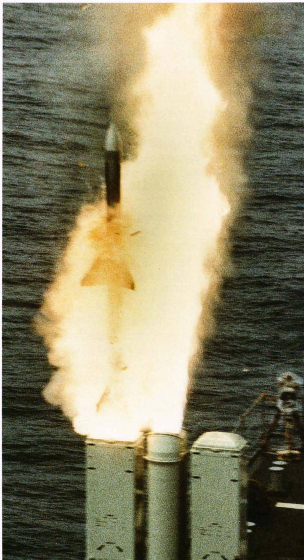
Figure 4. A NATO Seasparrow missile being launched from the Mk 48 Guided Missile Vertical Launching System on the USS Briscoe (DD-977) during at-sea tests.
