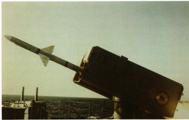
Figure 3. A NATO Seasparrow missile being launched from the Mk 29 trainable launcher on the USS Merrill (DD-976) during an exercise. Thirty-one ships of this class are outfitted with the NATO Seasparrow Surface Missile System.
