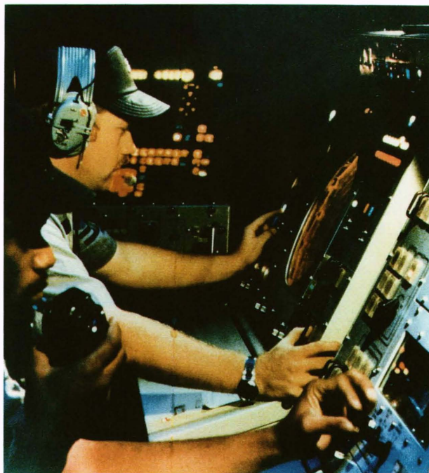
Figure 6. The Firing Officer (background) and Radar Set Console Operator (foreground) of the NATO Seasparrow Surface Missile System exercise positive control over Seasparrow engagements, and interact with automatic processes to make weapon direction and engagement decisions.
