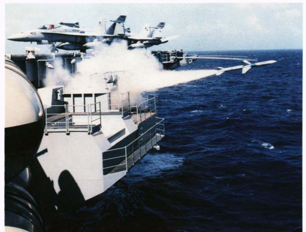
Figure 5. A NATO Seasparrow RIM-7M missile being fired from the USS Abraham Lincoln (CVN-72) in January 1990. All aircraft carriers are provided with Seasparrows.
