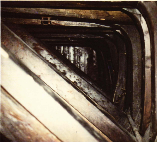
Figure 6. Photograph of the Fram 's internal bracing (taken by author). Compare with the "transverse section amidships" shown in Figure 4.
