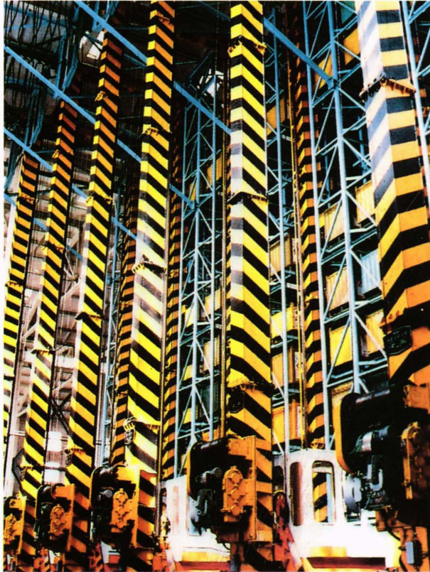
Figure 8. Computer-controlled warehouse automated to access high-bay areas.
