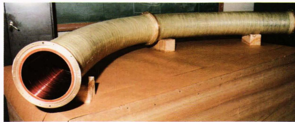
Figure 11. S-band sheathed-helix waveguide bend.
