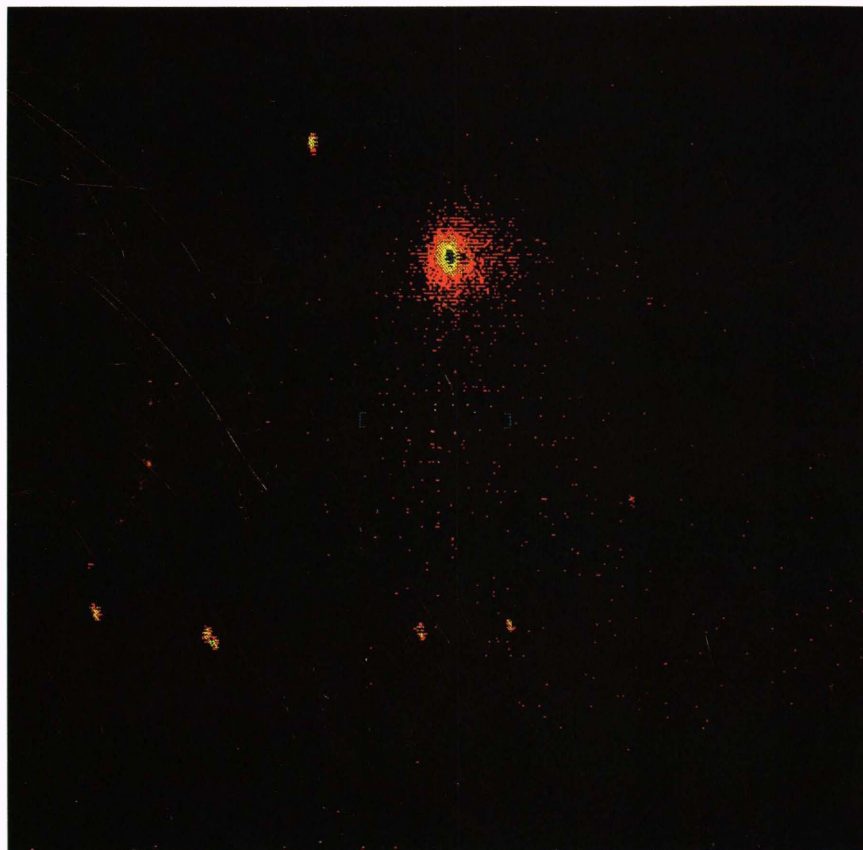
Figure 2. The Hopkins Ultraviolet Telescope television camera captures an image of Comet Levy. The rectangular area in the center is a 9 \times 116 arc second spectrograph aperture. The telescope was pointed so that the spectrum of a portion of the comet's tail could be measured. The comet's nucleus is shown above the spectrograph aperture. The nucleus has a brightness of 12 visual magnitude per pixel. The observation was made at an angle to the Sun of 43^\circ . The image was composed by adding two 0.5-s frames of the television camera output. (Photograph courtesy of the Johns Hopkins Center for Astrophysical Sciences.)
