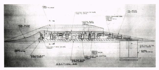
Figure 9. The external expansion ramjet (ERJ-2) model.
