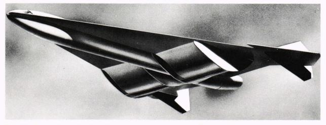
**Figure 15.** The principal configuration of the APL hypersonic transport was a 175-foot-long delta-winged aircraft with a wing span of 102 feet. It used turbojet engines to accelerate to Mach 3.6 and external expansion ramjets for propulsion at higher speeds, up to a cruise Mach number of 7. In the lower-speed range, the inlet ramps of the ramjet engine retracted to provide an opening for airflow to the turbojets.
