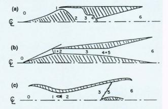
**Figure II.** Hypersonic ramjet forms. (a) Conventional ramjet. (b) Supersonic-combustion ramjet. (c) Standing-wave ramjet.
