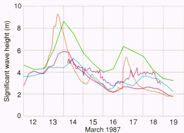
Figure 7. Twelve-hour wave height forecasts during LEWEX from four different numerical wave models, each using its own estimate of the wind field (WAM with ECMWF winds in red, ODGP with ODGP winds in blue, GSOWM with FNOC winds in green, and UKMO with UKMO winds in orange). Also shown are measurements from the Norwegian Wavescan buoy (in purple).
