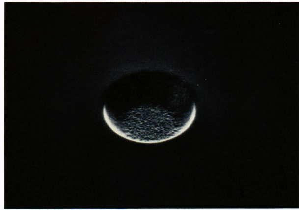
Figure 8. A round 50- \mu\text{m} -diameter via developed from 750- \mu\text{m} -thick (uncured) Probimide 348 photosensitive precursor.
