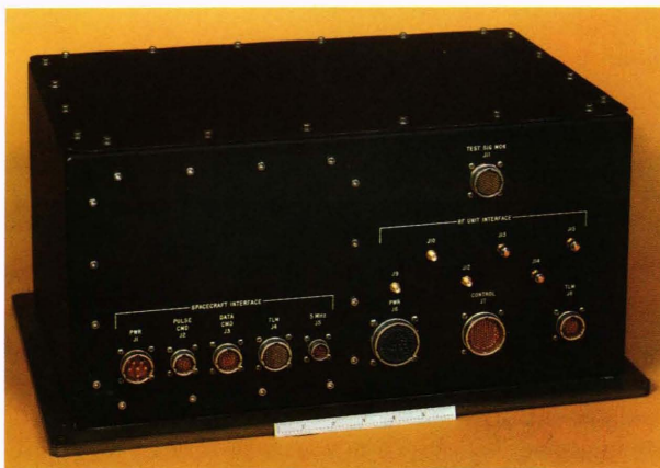
Figure 2. The Geosat-A signal processor. The design is an extension of that of Seasat-A, although it incorporates several major improvements.
