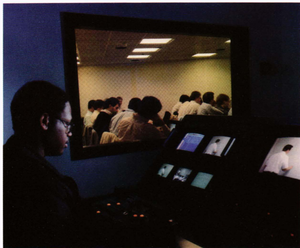
Figure 4 —The control room operator of the intercampus Instructional TV microwave link can control and monitor transmissions to other locations and to the students' desk monitors while operating the three video cameras available in the classroom.
