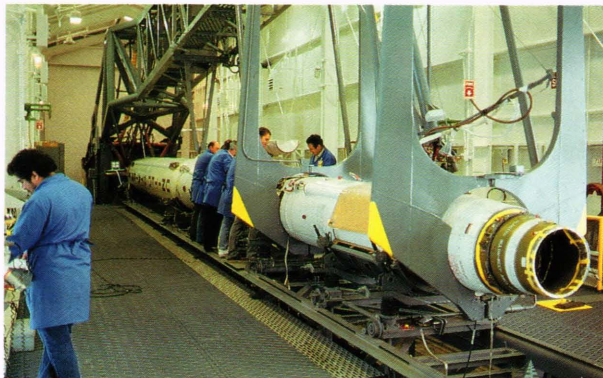
At the pad. Inside the mobile shelter, LTV engineers check out the 63-ft-long first three stages of the Scout rocket. The combined fourth stage and spacecraft will be mated at the open end.
