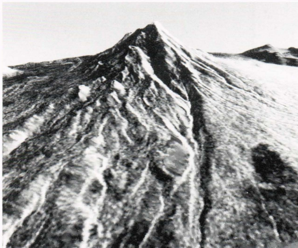
Figure 2 —Stereo images acquired by the SIR-B were used to generate topographic contours (top) and perspective views (bottom) of Mt. Shasta in California.
