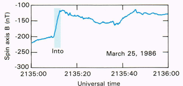
Figure 7 —A 1-minute segment of magnetic field data from the spin axis sensor (approximately in the east-west direction) over the morning auroral zone.
