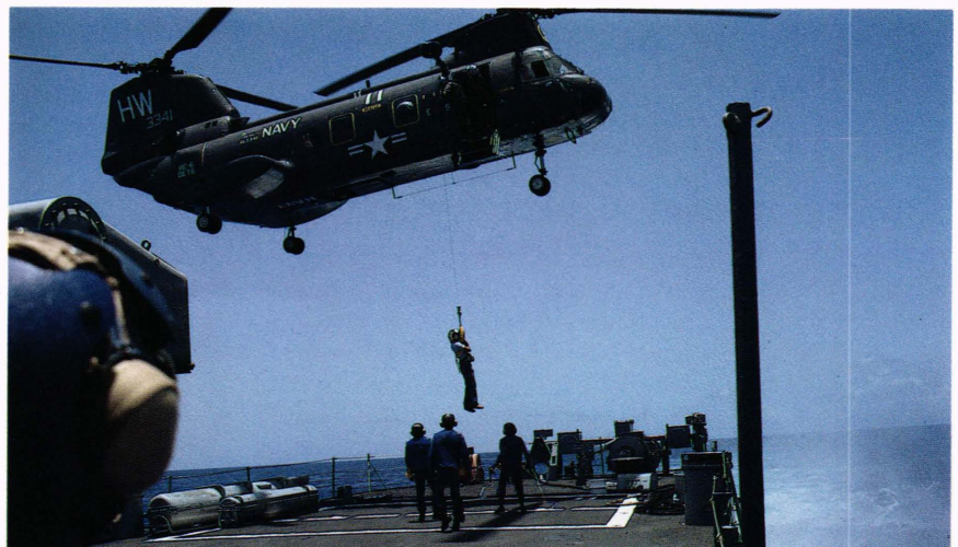
A civilian passenger descending by bridle from a CH-46 helicopter to the deck of USS Mahan (DDG-42).
