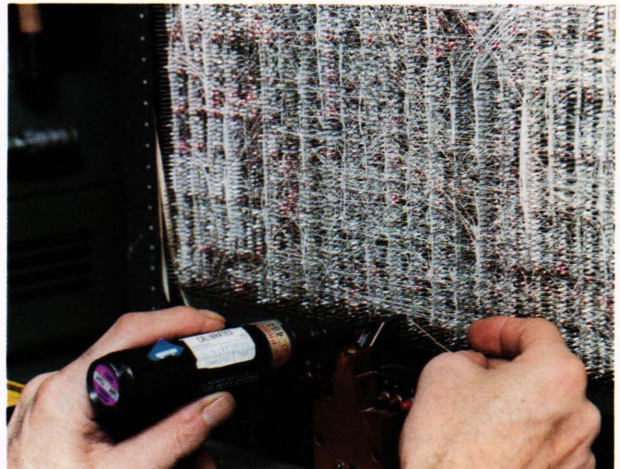
Figure 2 —(top) An operator performing semiautomatic wire wrap on a typical wire-wrap circuit board using the Gardner Denver system. (bottom) A wire-wrap tool in place prior to completing a wire wrap.
