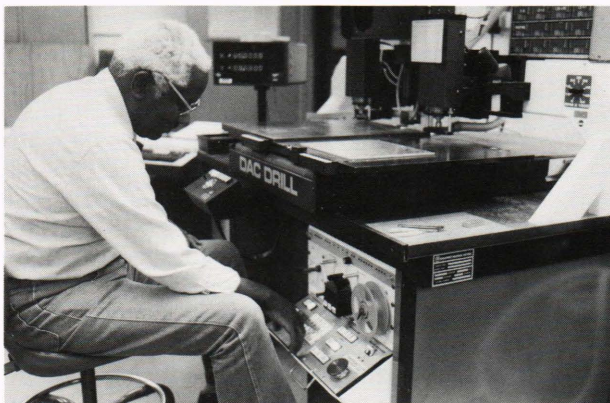
Figure 4—(left) An overall view of a CAD computer numerically controlled drill/router. (right) Example of material that has been drilled and routed by the DAC drill/router.
