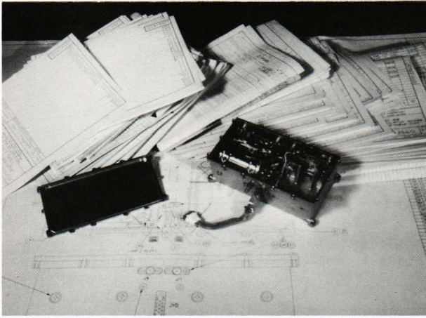
Figure 4 —The 5-megahertz dual oscillator unit and associated engineering drawings shown represent the typical amount of design information required to build such a common electronics unit at APL.
