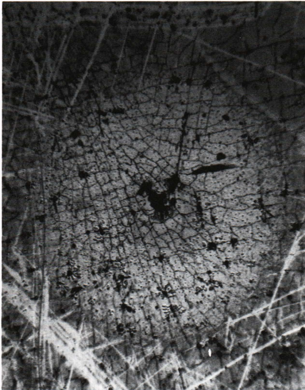
Figure 7 —Optical micrograph (30 power) of the eroded silver-coated Teflon surface. According to X-ray analysis, only a small amount of silver remains in the heart of the eroded area. Many degradation cracks are observed in the Teflon in the sun-illuminated area.
