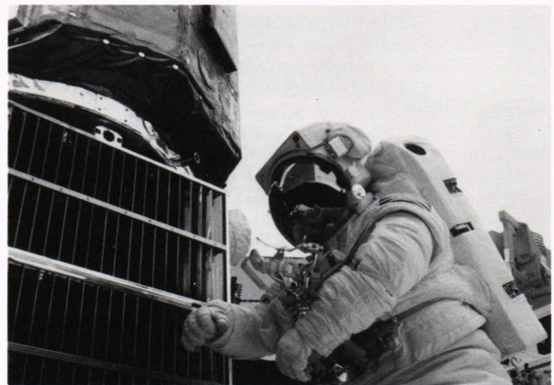
Figure 1—An astronaut repairs Solar Max, replacing sections to be returned to earth. (Photograph courtesy of NASA.)
