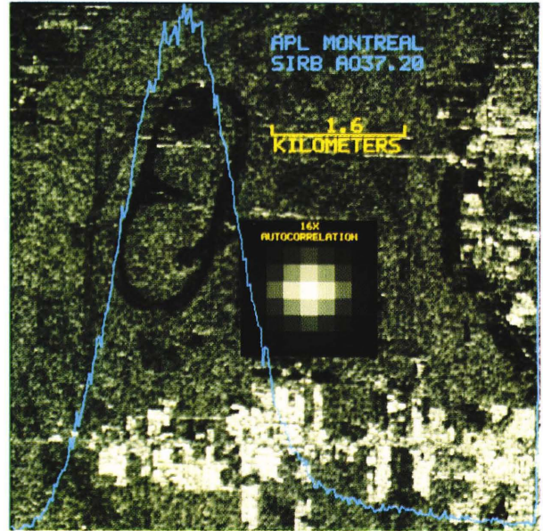
Figure 15—Detail from Fig. 14, also showing processor resolution and sidelobe structure as measured by noise autocorrelation.
