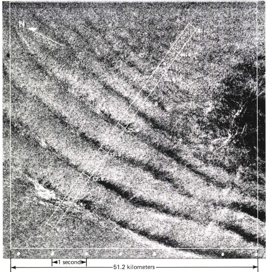
Figure 3 —L-band radar image from SIR-A taken November 11, 1981, near the Andaman Islands, showing a packet of 6-kilometer-long solitons and what is thought to be a rain squall. Dimensions are 51.2 by 51.2 kilometers. (Photograph courtesy of the Jet Propulsion Laboratory.)
