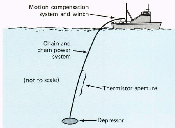
Figure 4—A schematic of the APL high-density towed thermistor chain used to acquire these data.
