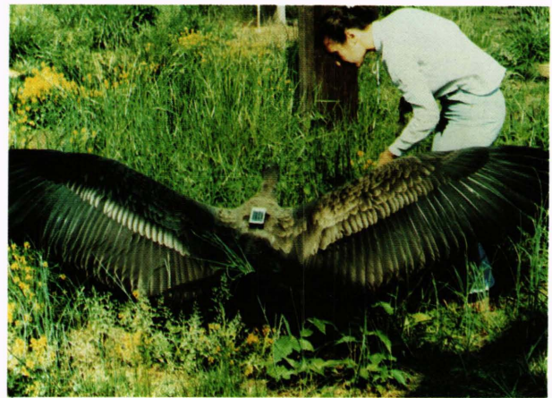
Figure 5 —Test of the solar power design with a captive subadult Andean condor at the Patuxent Wildlife Research Center. The bird wore a small plastic box containing a solar array, batteries, charge control circuitry, a battery load, and a small transmitter to indicate whether the batteries were charged. The test provided valuable data on the amount of sunlight received under more realistic conditions than laboratory tests. The small transmitter in the package also provided temperature data needed for the design of the crystal oscillator of the satellite transmitter. The bird tended to keep the temperature in the box regulated within a 20°C range.
