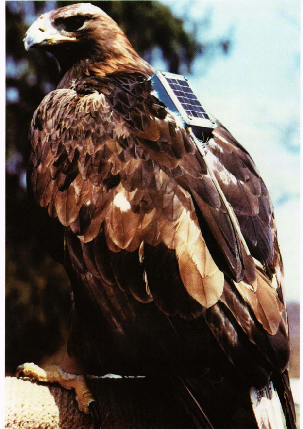
Figure 10 —The first Argos bird transmitter on a captive golden eagle for field tests. The bird wore the transmitter for five weeks and provided information on accuracy, solar powered design, and bird adaptation.
