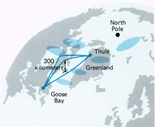
Figure 16 —Schematic view of the Thule-Goose Bay propagation experiment showing the manner in which ionospheric electron density enhancements (represented by the shaded regions) produce multipath ionospheric propagation between the two stations.
