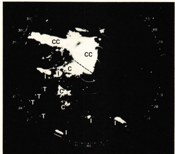
Figure 8—Plan position display of raw radar video from the sea surveillance experiment. The display covers 70 nautical miles showing the Channel Islands (I) and the coast of California (CC). Close-in sea clutter (C) and some long-range targets (T) are visible.
