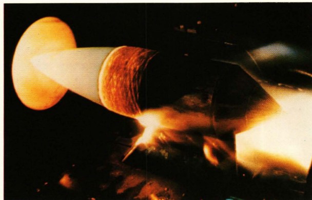
Figure 5 – A missile radome test under conditions that simulate a Mach 8 flight indicates the severe aerodynamic heating at hypersonic speeds. Other missile components such as leading edges are also developed in ground test facilities.
