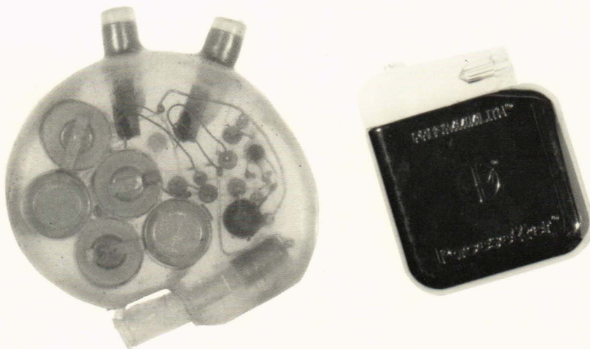
Figure 1 — Comparison of a fixed-rate pacemaker (circa 1970) and a recent, multiprogrammable, demand pacemaker.
