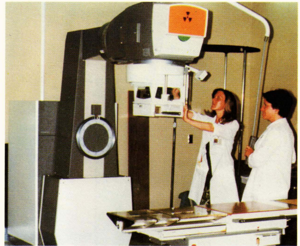
Figure 9 — The Siemens Gammatron cobalt-60 machine. Technologists are setting up the machine for patient treatment by preadjusting beam collimators.
