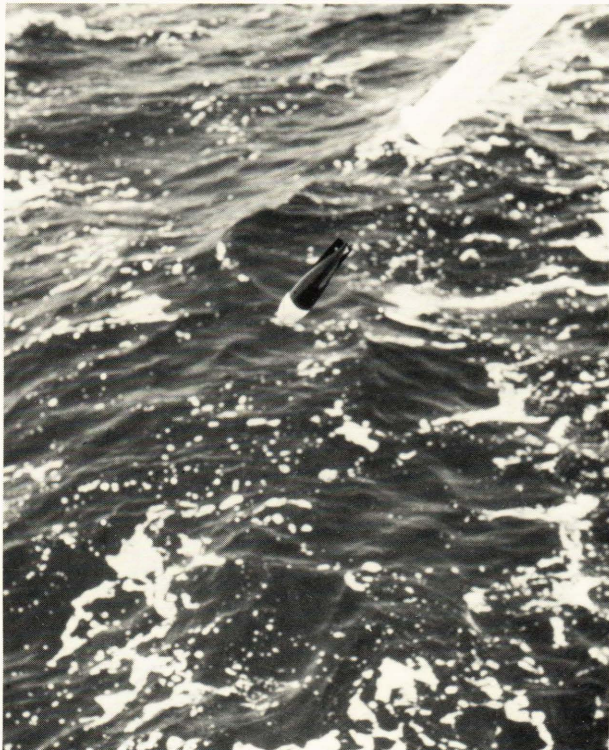
Figure 5 — An expendable bathythermograph probe immediately after launch. Notice the very fine wire, trailing from the probe, over which data are transmitted to a recorder. In contrast to the sound velocimeter shown in Fig. 4, these probes can be launched from a moving ship.
