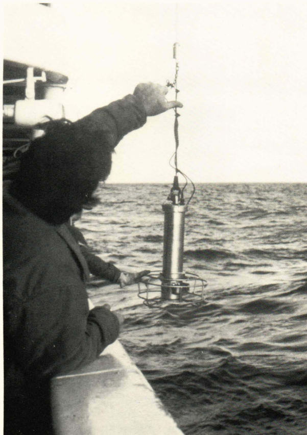
Figure 4 — The Navy oceanographer aboard the USNS DeSteiguer prepares to lower a sound velocimeter. This instrumentation package measures the speed of sound directly as a function of depth and also measures temperature and salinity.
