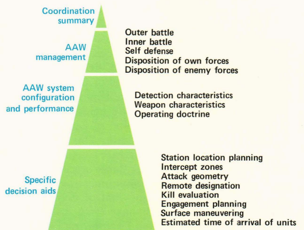
Figure 4 — Displays are made available to the Commander according to a tiered information structure that allows selection of displays to give him complete knowledge of the tactical situation, anti-air warfare (AAW) system capabilities and status, and access to specific decision aids for key problems.
