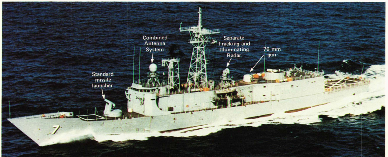
Fig. 2 —USS Oliver Hazard Perry (FFG-7), commissioned in December, 1977, was the first ship of a class of about 50 to be built. This 3600-ton ship, with a complement of 11 officers and 153 enlisted men, provides protection for underway replenishment groups, amphibious forces, and military and mercantile shipping.
