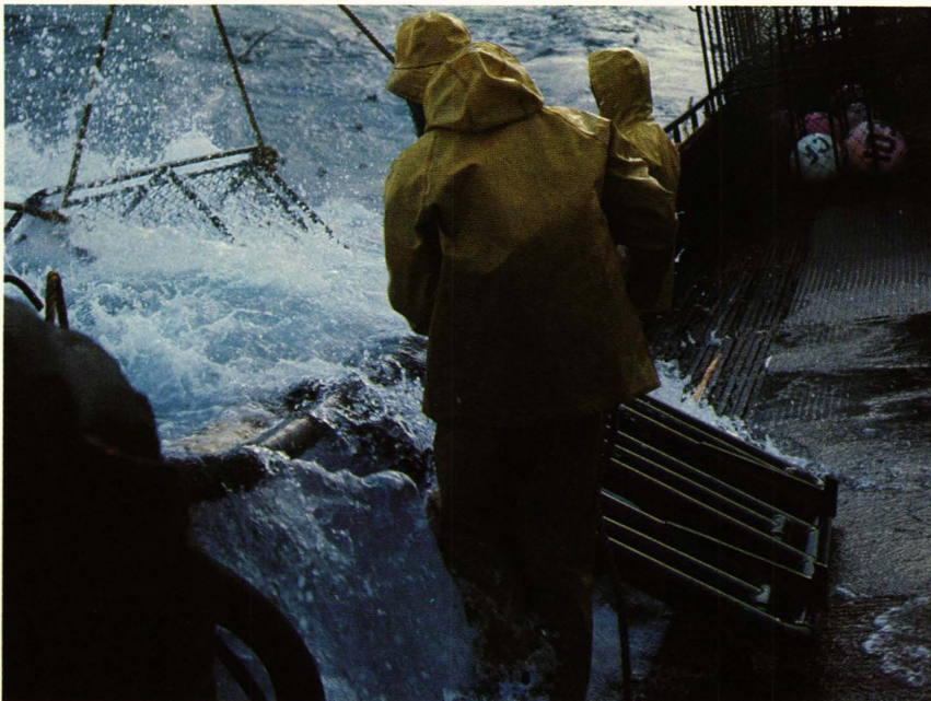
Up from the Bering Sea churns a crab pot of steel frame and nylon mesh, 7 × 7 × 3 feet, weighing 700 pounds empty but at least another 1000 pounds more if full of king crabs. The pot will be rested at a tilt on the hydraulic launcher (lower right). Astern are other pots with buoys and lines stored inside.*
