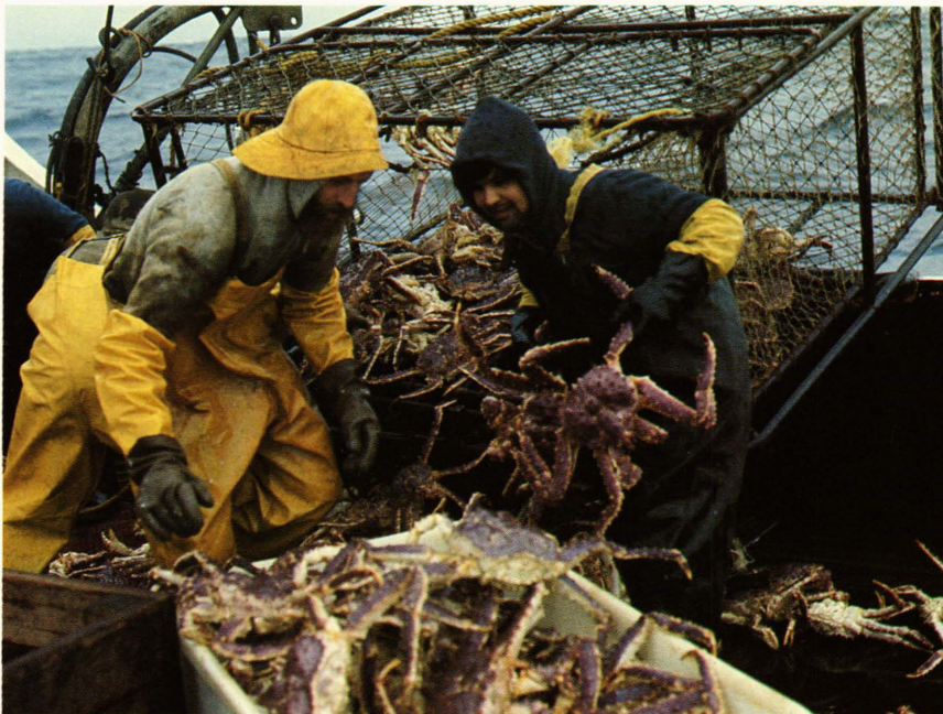
Working on the run as a team, a four-man crew removes 7- and 8-pound king crabs and rebaits a huge crab pot. The complete cycle between appearances of pots at the rail takes 3 to 5 minutes. The pace would not be possible without the hydraulic crab block (shaft above deck, left), which raises the pot from the seafloor 60 fathoms below in about 1 minute while automatically compensating for slacks and tensions on the line caused by the boat's motion in heavy seas.
