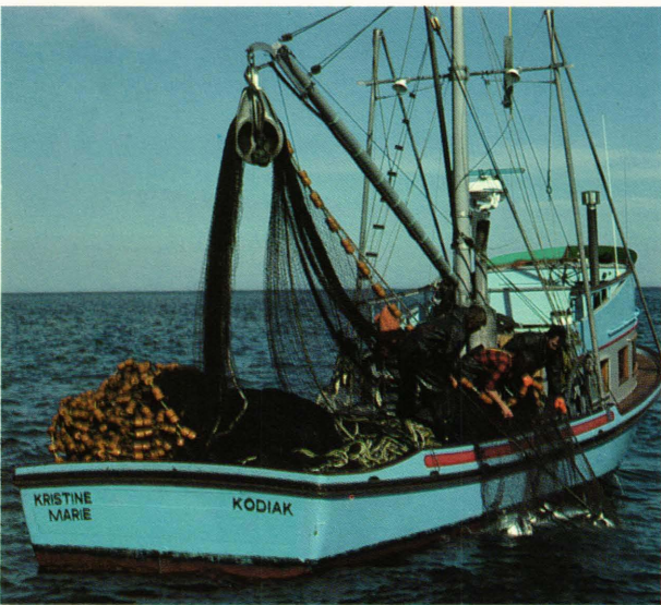
Different hydraulic power blocks handle large and small seines. In the top photo, the crew of a herring seiner out of Gloucester, fishing through the night while the herring rise to feed, brings in a net several times the size of that on the Alaskan salmon seiner (bottom). In both instances the heaviest work of hauling aboard the wet net, corks, and leaded line is accomplished by the hydraulically operated power block suspended from the boom. Before the power block was introduced in the mid-1950's, it required more crewmen far longer to perform the same work. On the Alaskan seiner note the radar antenna above the wheelhouse. Boats of this size did not have radar until affordable transistorized versions appeared on the market in the mid-1960's.
