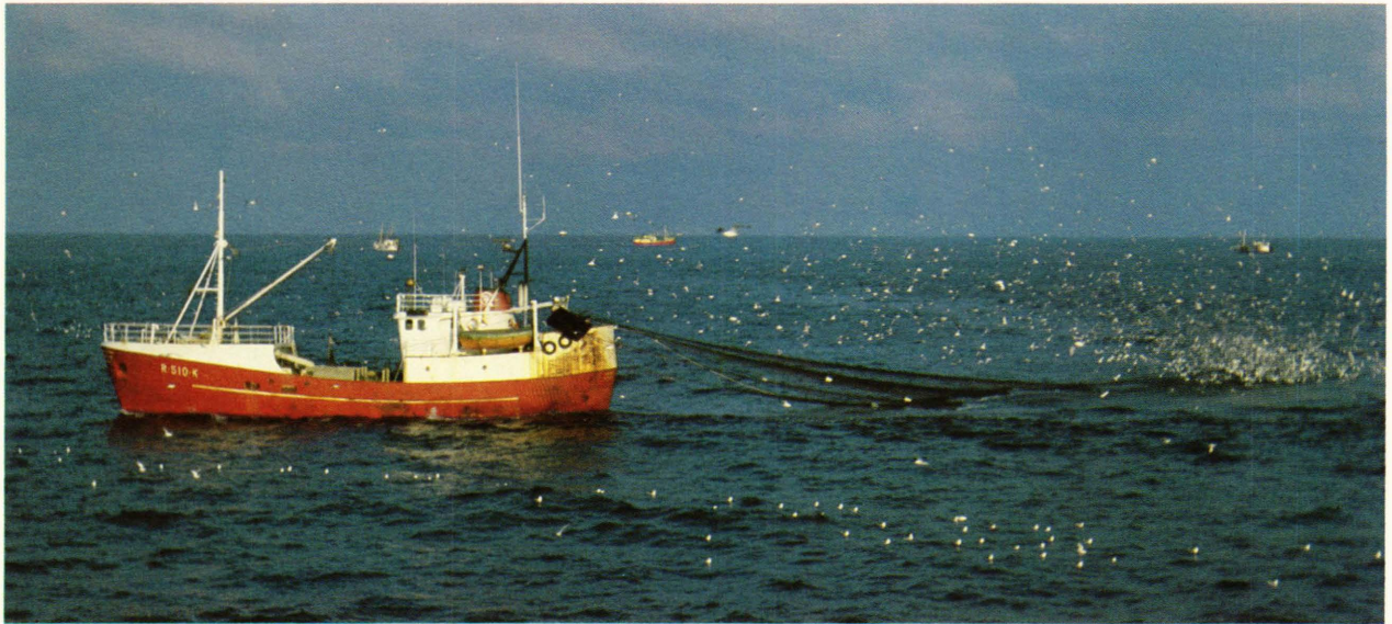
Norwegian trawlers patrol the far northern capelin grounds between Norway and the Soviet Union with nets raised, ready to lower quickly for a set if the echo sounder reveals a school of fish below.
