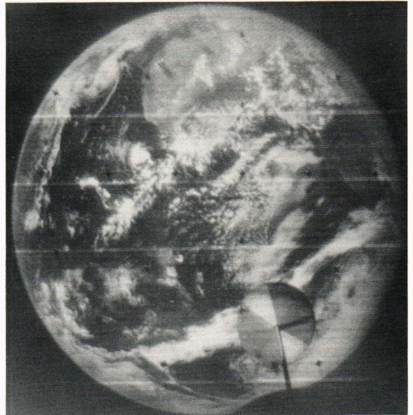
Fig. 2—Photograph of the earth taken by the TV cameras of the DODGE Satellite. The circular object in the bottom of the picture is a sectored sphere, mounted on the satellite, that is used for color calibration studies.
