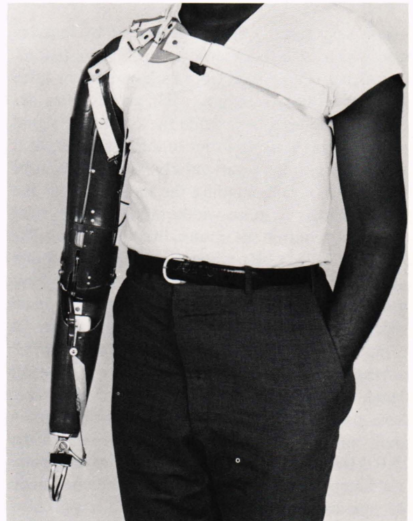
Fig. 3—Above-elbow prosthesis with power unit in the elbow and battery pack on the belt.
