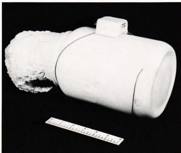
Fig. 5—Photo of the “Plastic Swan” which is the electrical equivalent of a Whistling Swan.
