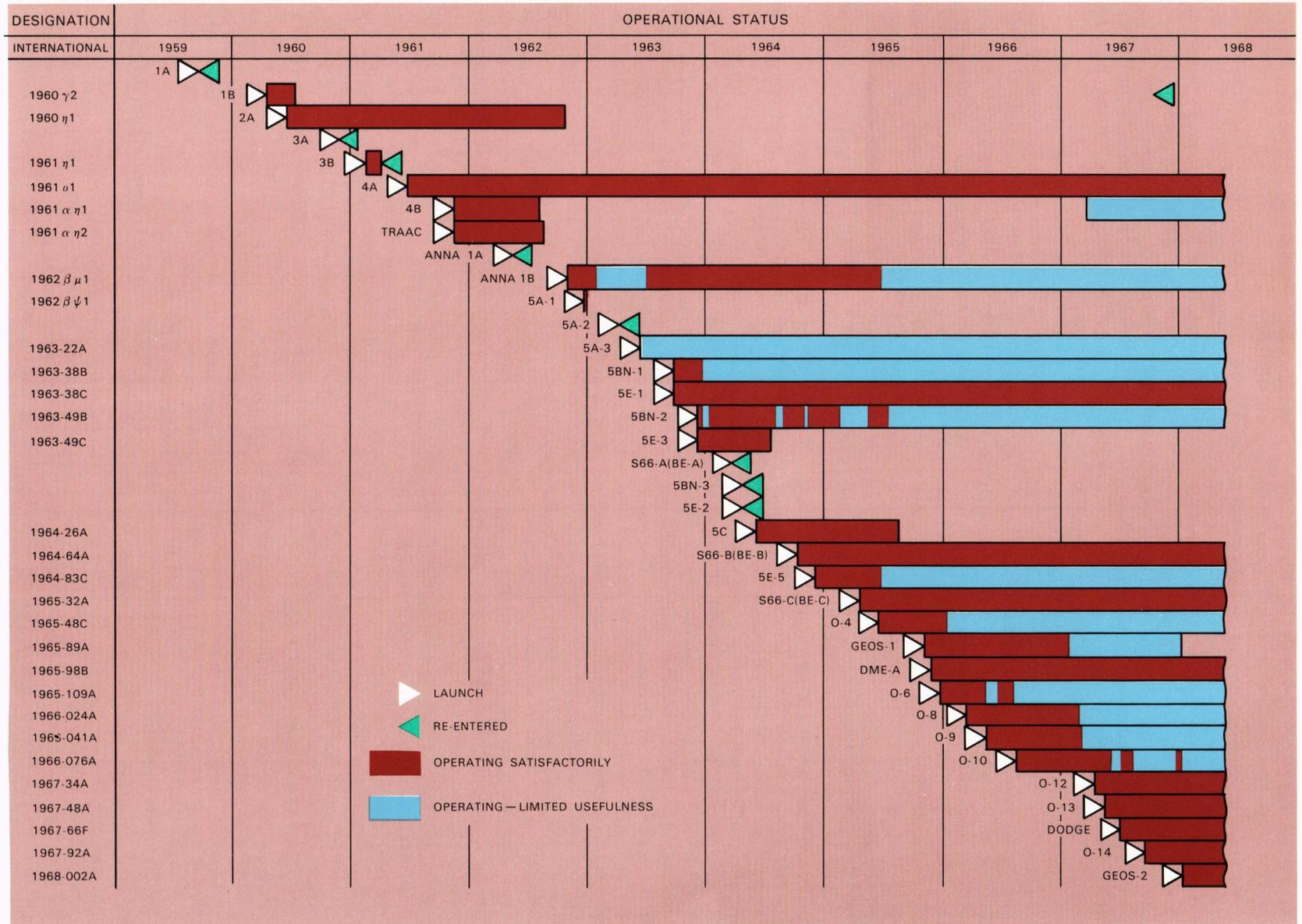
Fig. 2 — Operational Status History of the 36 Satellites Fabricated at APL.
