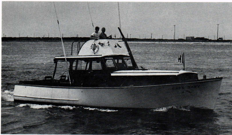
Fig. 2—A 35-foot Jersey sea skiff, Cap's Baby . This cruising boat is comfortable and stable, though not as highly styled as some.
