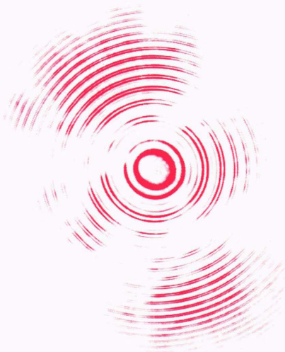
Fig. 10—An interference pattern from a Fabry-Perot interferometer, showing a feedback effect.
