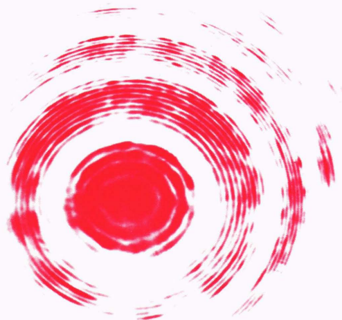
Fig. 7—An interference pattern from a Fabry-Perot interferometer. The laser was in a confocal configuration, and the plate separation of the interferometer was 17 cm.
