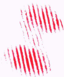
Fig. 6—An interference pattern from a Jamin interferometer. Note the position of the fringes in the region between the transverse mode parts.
