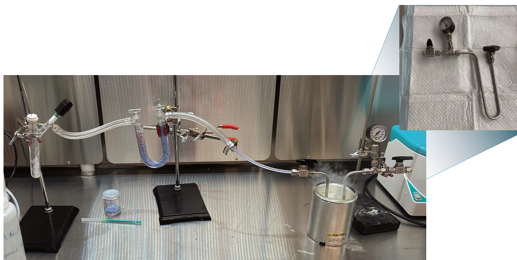
Figure 2. The apparatus used to purify xenon from \text{XeF}_2 . Inset, the U-tube fitted with a pressure gauge and valves on either end containing cryotrapped xenon.
