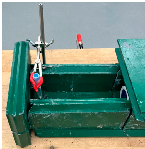
Figure 12. An example of the HPGe \gamma counting setup. The HPGe, shown on the right side of the image, is housed in lead bricks.
