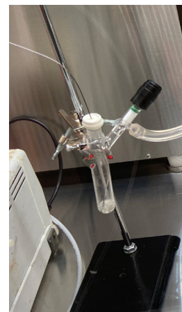
Figure 3. Removal of dissolved xenon gas by sparging \text{XeF}_2 dissolved in 1N NaOH with gaseous nitrogen.
