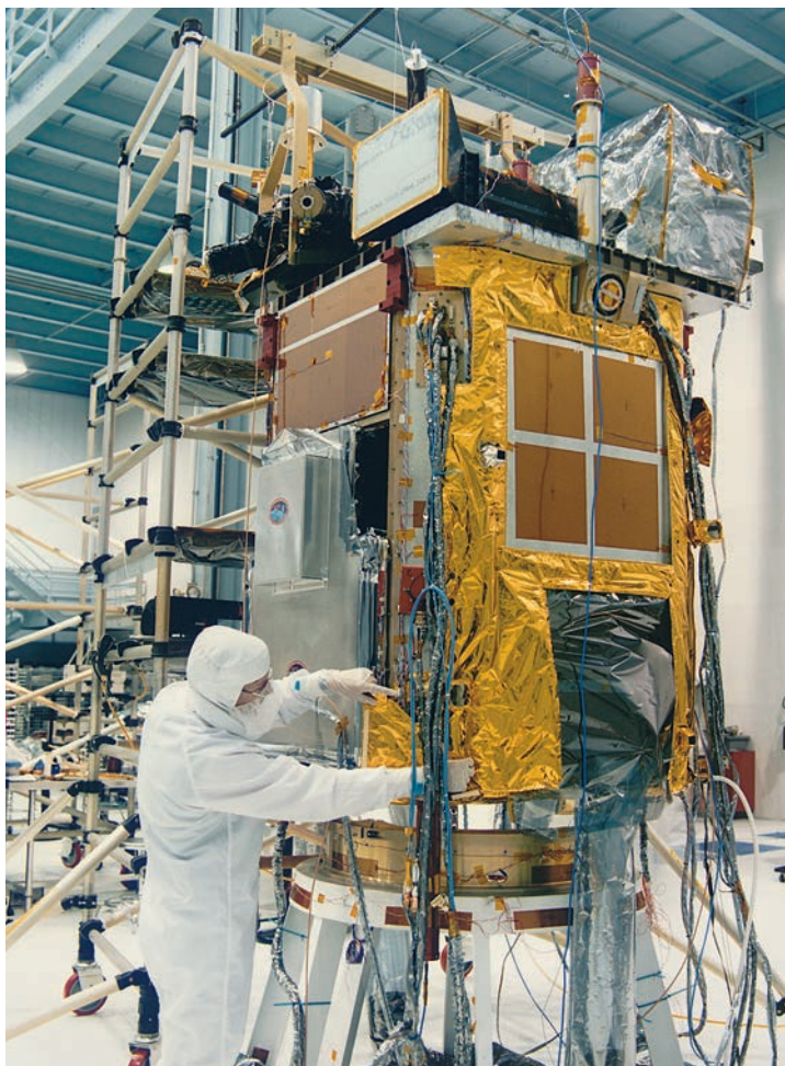
Two of four telescopes on the Doppler Interferometer instrument were evident here on NASA's TIMED spacecraft, launched in 2001.
