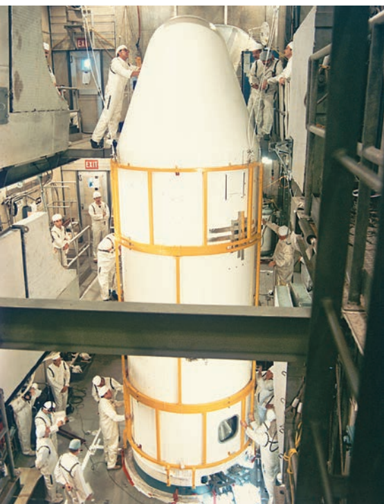
By the time Delta 181 was enclosed in its fairing, only personnel from McDonnell Douglas were permitted to accomplish the task as APLers watched. The fairing is almost as fragile as an eggshell, and generous use of duct tape—known as “hundred-mile-an-hour tape” in the space community—helped to keep out contaminants. Delta 181 launched on February 8, 1988.
