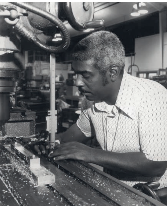
Precision tools operated by expert hands have been a distinction of APL's shops from its earliest days. Employees like Vernon Nash built long and productive careers running machines like this Hydrotel, which traced prototype parts made by machinists.
