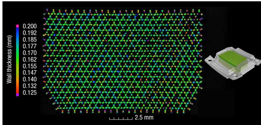
**Figure 4.** Challenges with validation. Traditional measurement tools in the XRCT software could generate simple wall thickness measurements of the collimator geometry but, because of the wide range of hole orientations, they could not be used to quantifiably check the alignment of the final holes, the number of blockages within the tubes, or the integrity of the walls.
