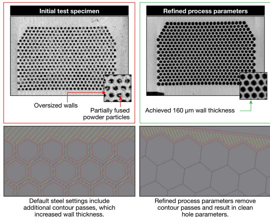
**Figure 2.** Steel settings and resulting prototypes. Left, default steel settings (bottom) included two contour laser passes in addition to an infill operation, which resulted in oversized walls and a large number of blockages. Right, by tuning the input parameters (bottom), the team limited the walls to a single laser pass, resulting in thin walls and no blockages.
