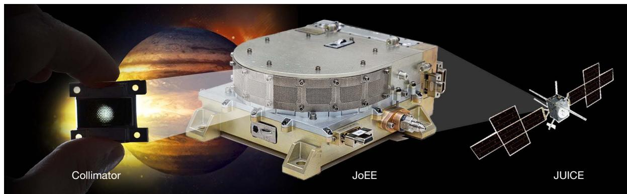
**Figure 1.** The JoEE spectrometer, part of the PEP-Hi instrument. The spectrometer (center) has strict requirements on collimation of electrons to measure their angular distributions in the harsh Jovian radiation environment onboard JUICE (right). APL solved that challenge by using AM to fabricate robust and precise collimators (left).
