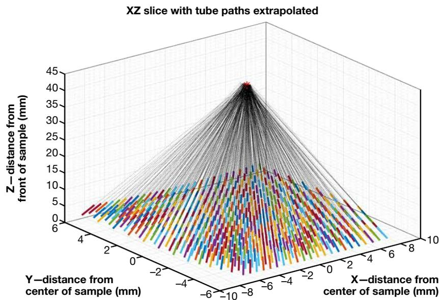
**Figure 5.** Validation solution. By combining the simulated viewpoint of the instrument with image analysis tools, the team was able to individually fit each hole pattern and calculate the focal point of the collimator pattern.
