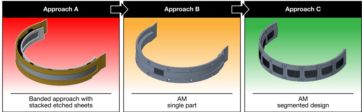
**Figure 3.** Approaches to collimator manufacturing. While the ultimate shape of the collimator remained the same, APL’s scientists, engineers, and machinists had to rapidly iterate to find a design that could be readily manufactured.
