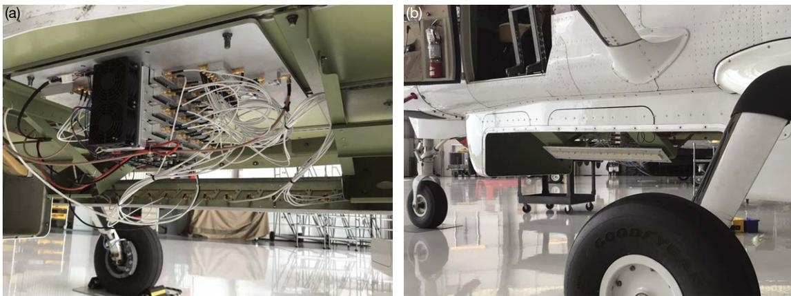
**Figure 24.** FMPA installation into the hold of a Cessna Caravan. (a) The electronics assembly and (b) the 16:1 linear antenna array.
