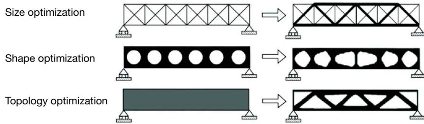
**Figure 5.** Comparison of optimization methods. As the terms suggest, size optimization involves optimizing an object's size, and shape optimization involves identifying the optimal shape of the object or its openings. Topology optimization involves optimizing the object's geometry and therefore encompasses size and shape optimization. (Image reprinted from Gebisa and Lemu, Attribution 3.0 Unported, CC BY 3.0, <https://creativecommons.org/licenses/by/3.0/>)
