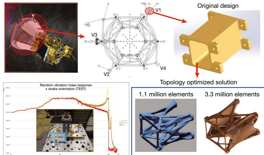
**Figure 7.** Optimization cycle of the PSP bracket. Top (left to right), rendered image of PSP, locations of the bracket of interest on a drawing of the spacecraft truss system, and bracket design that flew (unoptimized). Bottom (left to right), the vibration test setup overlaid on a simulation and measured response plots and CAD images of topology-optimized solutions.
