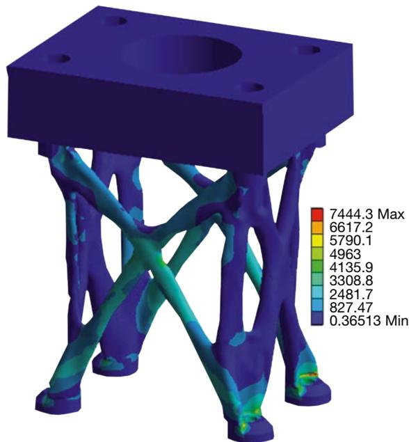
**Figure 8.** FEA results validating the PSP bracket optimization. Topology optimization reduced the bracket's weight by 65%.
