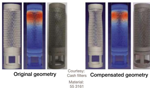
**Figure 9.** AM print process simulation of original and compensated geometry. Red shows locations of high distortion. (Image reprinted with permission from Ansys.<sup>12</sup>)
