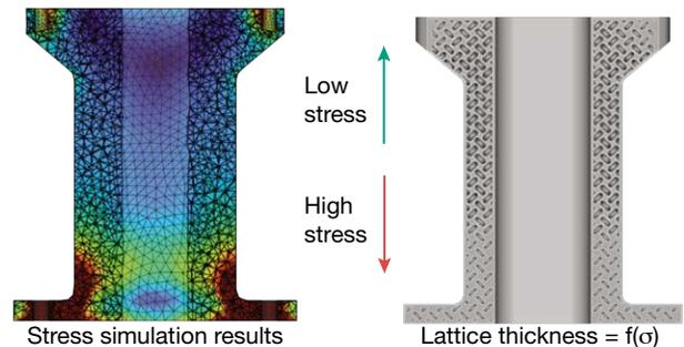
**Figure 4.** Example of architected cellular structures designed with implicit modeling. The characteristics of the cellular structure (i.e., lattice) are varied throughout the bracket, enabling location-specific characteristics similar to those found in nature.
