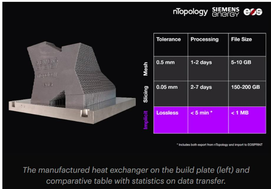
**Figure 10.** The heat exchanger produced with Implicit Interop capability demonstrates the capability of going from nTop to the EOS Slicer in under 5 minutes with under a megabyte of data. (Reprinted with permission from nTop.)
