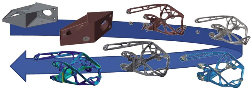
**Figure 6.** Example of topology optimization cycle. The bracket design evolved from a simple CAD drawing to a fully optimized design.
