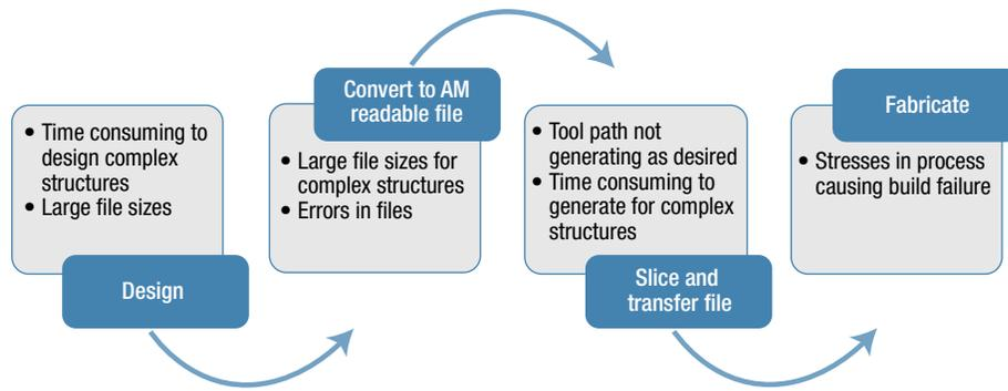
**Figure 1.** AM challenges. The AM workflow is a feedback loop, so a challenge at any one stage could require a part redesign, a change in processing, a different method of modeling entirely, or all of these. Such time-consuming changes negate the main benefits of AM—rapid iterations and quick turnarounds.
