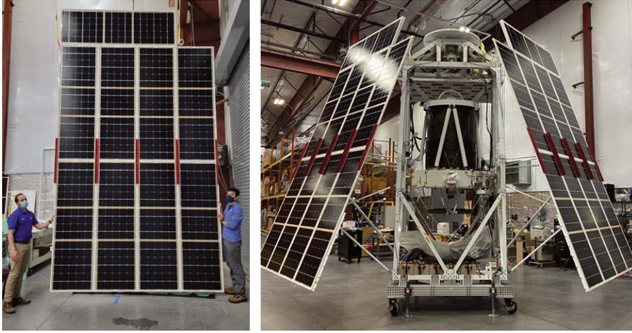
**Figure 12.** One of two GUSTO arrays. These high-efficiency panels are key to recharging the high-capacity batteries on GUSTO's planned 75-day mission.
