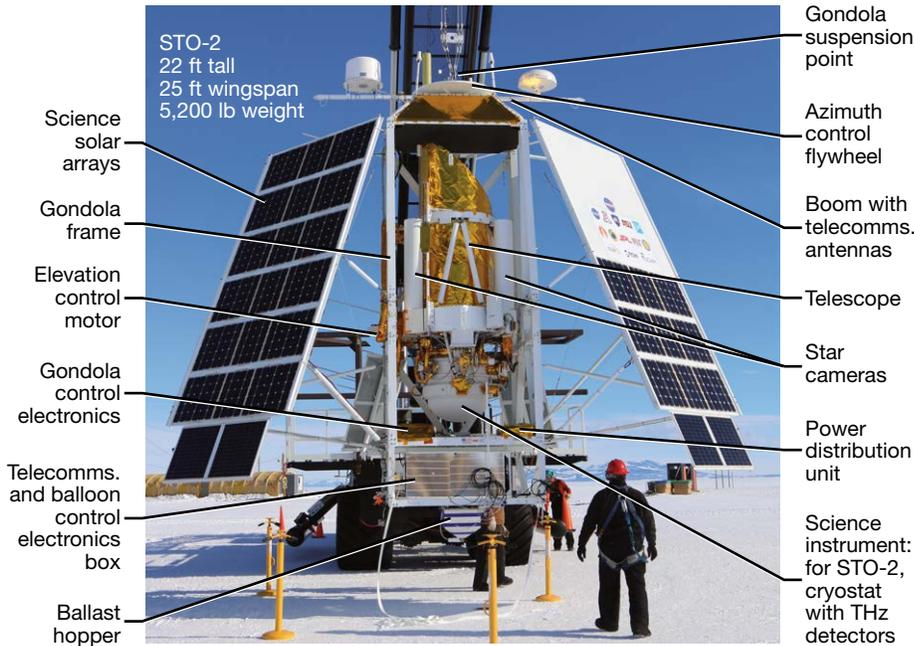
**Figure 2.** Anatomy of a balloon gondola. The gondola supports telescopes and other scientific equipment. This gondola from the second Stratospheric Terahertz Observatory II (STO-2) mission is 22 ft (6.7 m) tall and weighs 5,200 lb (2,358 kg). It houses solar arrays, telescopes, and other equipment necessary to power and control the scientific instrumentation.
