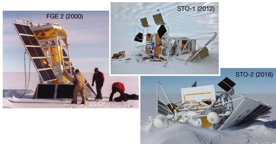
**Figure 18.** Landings of three APL balloon gondolas in Antarctica. The goal is a soft (i.e., snowy) landing so that the gondola remains mostly in one piece and data storage and other components can be easily recovered.
