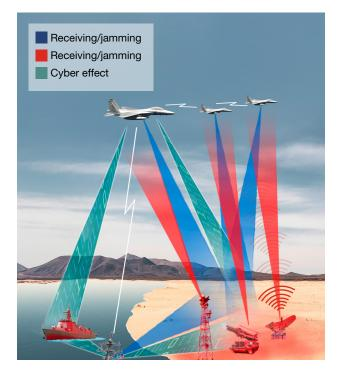
**Figure 5.** Integrated EW and cyber fires concept example. Distributed Blue platforms collaboratively perform ES and deliver EA and cyber effects against Red threat systems.
