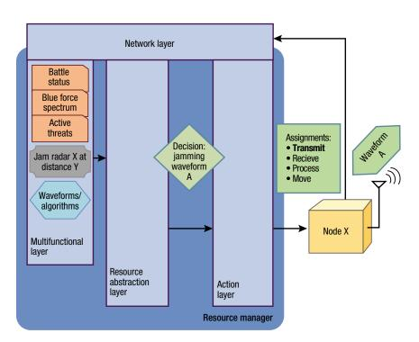
**Figure 10.** Using the SAD and objectives, the resource manager directs node X to broadcast waveform A to complete the objective.
