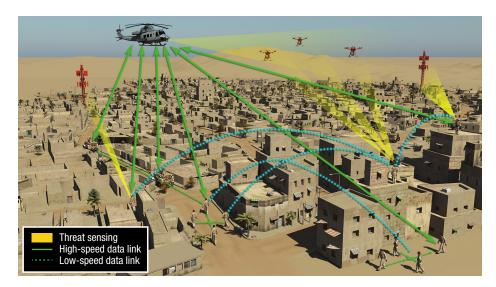
Figure 2. A ground EW network. In this scenario, vehicles, body-worn systems, and a helicopter must interact to better engage existing cellular networks and adversary unmanned aerial vehicles.
