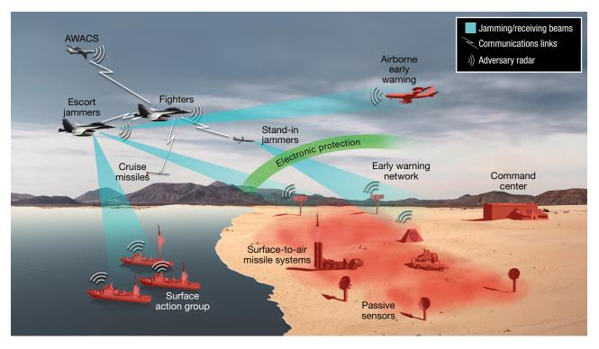
Figure 1. An airborne EW network. This diverse network engages naval and ground radar and surface-to-air missile assets. AWACS, airborne warning and control system.
