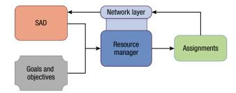
**Figure 3.** Resource management architecture's inputs and outputs. The backbone of the resource management architecture, the network layer moves information to and from nodes and the resource manager and adopts the OSI model to allow for flexible design when creating connections between EW platforms.
