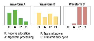
**Figure 7.** RAPD resource trade-offs between waveforms. In multiple target scenarios, RAPD outputs would be weighted against one another, the resources available, and the priority of the target to determine an optimal output that would satisfy mission needs.
