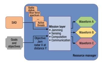
**Figure 6.** Overview of the mission layer and potential outputs. The SAD checks battle status to verify the authority to engage and then selects the jamming waveform among waveform A (most optimal), waveform B (optimal), or waveform C (less optimal),
