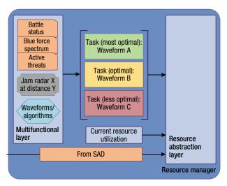
**Figure 9.** The resource abstraction layer taking all provided inputs to provide a final decision to the action layer. The layer configures the action layer to execute waveform A (i.e., configure the sensing, processing, and transmit resources).
