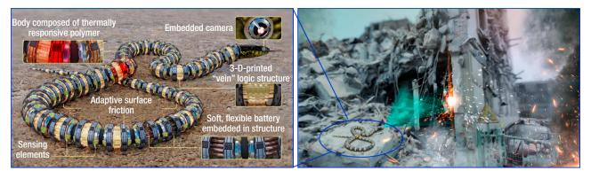
**Figure 4.** The robosnake. The vision for a soft, untethered robosnake integrates a variety of technologies and can be used for both Department of Defense and civilian applications.
