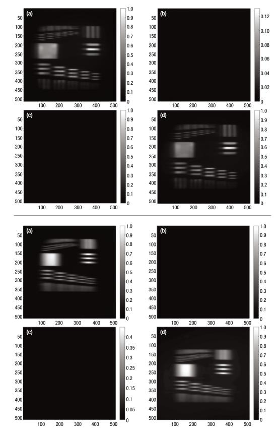
**Figure 3.** The images captured. Images of the 4.26-µm (top four panels) and 4.67-µm (bottom four panels) reflected from the metalens associated with the following polarization sequences: (a) TE input, TE detect; (b) TE input, TM detect; (c) TM input, TM detect; and (d) TM input, TE detect.
