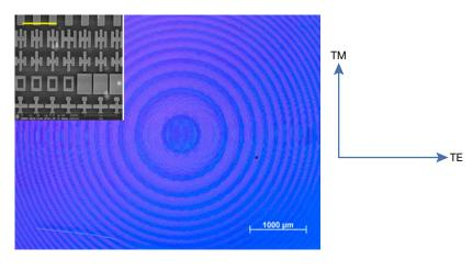
**Figure 1.** Optical micrograph and SEM images from the 1-cm-diameter metalens. The yellow scale bar in the SEM image is 3  $\mu$ m in length. The TM and TE polarization designations are shown on the right.
