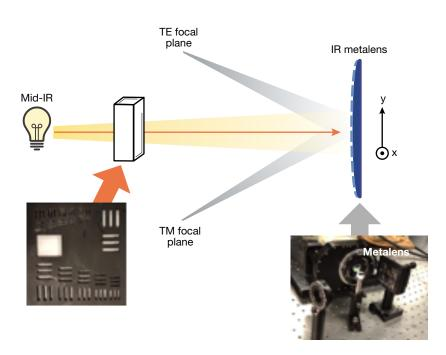
**Figure 2.** Illustration of the mid-IR metalens's performance when illuminated by an unpolarized source. Under this sample orientation, the two different states of linear polarization are deflected and imaged to the TE and TM focal planes. The actual metalens is shown on the right side.
