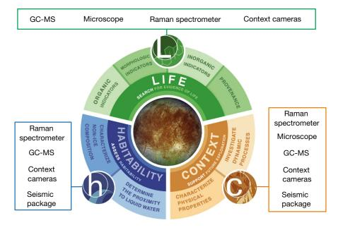
**Figure 8.** Europa Lander concept science goals and strawman instrument payload. The science of the Europa Lander mission concept focuses on searching for biosignatures in Europa's near subsurface through collecting and analyzing several ice samples from >10 cm depth and assessing habitability and contextual information with in situ techniques. GC-MS, Gas chromatograph–mass spectrometer. (Based on a NASA image from Hand et al.<sup>28</sup>)
