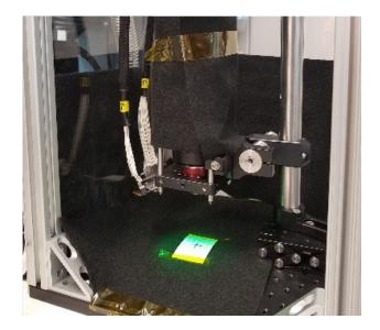
**Figure 4.** Prototype version of the Advanced Multispectral Infrared Microimager (AMIM) instrument. The instrument is shown with green (525 nm) LEDs turned on.
